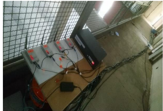
Figure 10. Hardware components: VR glasses and batteries (on the left), and switch and receivers (on the right).
