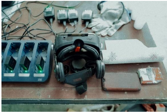
Figure 10. Hardware components: VR glasses and batteries (on the left), and switch and receivers (on the right).
